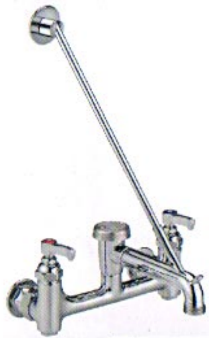
Model 4201C Two-Handle Sink & Pantry Faucet Heavy Duty Assembly With Vacuum Breaker 1/2" Npt Inlets Pail Hook and top Brace Build in Stop Device With Screwdrive Slot Provides Sparate Shout-Off for each Valve
